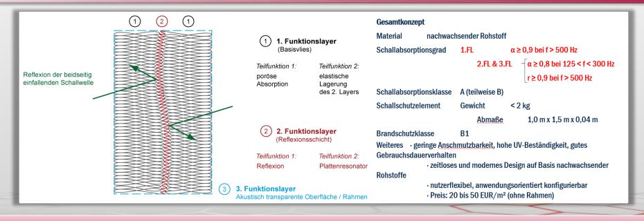
Development of elements with low thickness for the absorption of preferably low-frequency sound waves on the basis of nonwoven structures for the overall improvement of offices
